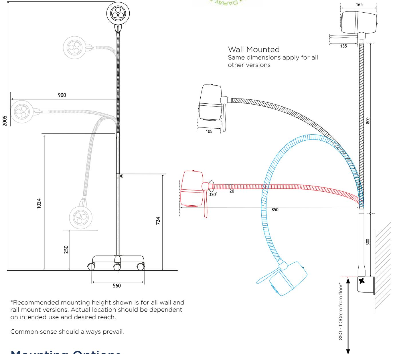
\*Recommended mounting height shown is for all wall and rail mount versions. Actual location should be dependent on intended use and desired reach.
