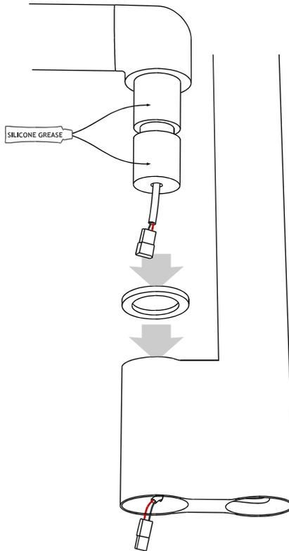
Join the connector from the primary arm to the connector from the down-tube.
