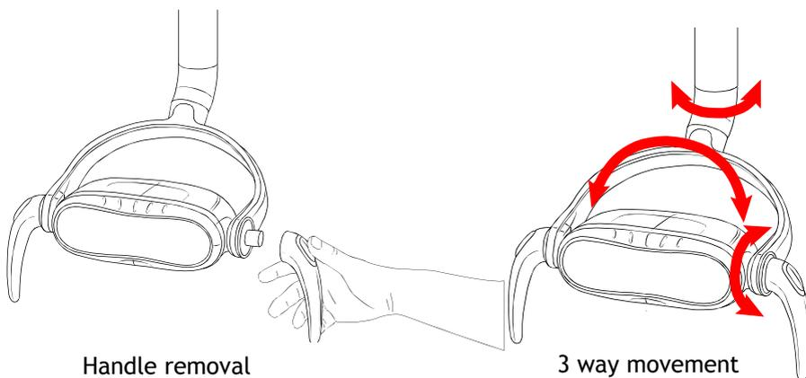
**Note: The handles are removable for cleaning but are NOT suitable for autoclaving**
