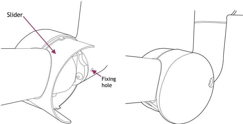
2. Align holes in cover and painted elbow. 'Nip up' the screw to secure.
