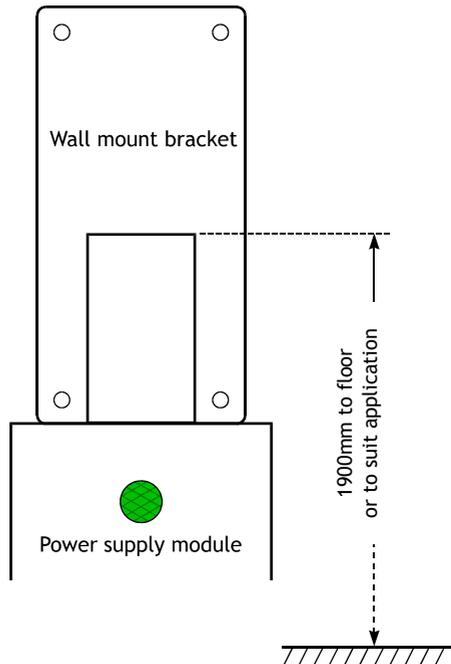
The power-supply module requires an earthed 230V AC electrical supply either fed into it via a switched fused spur.
